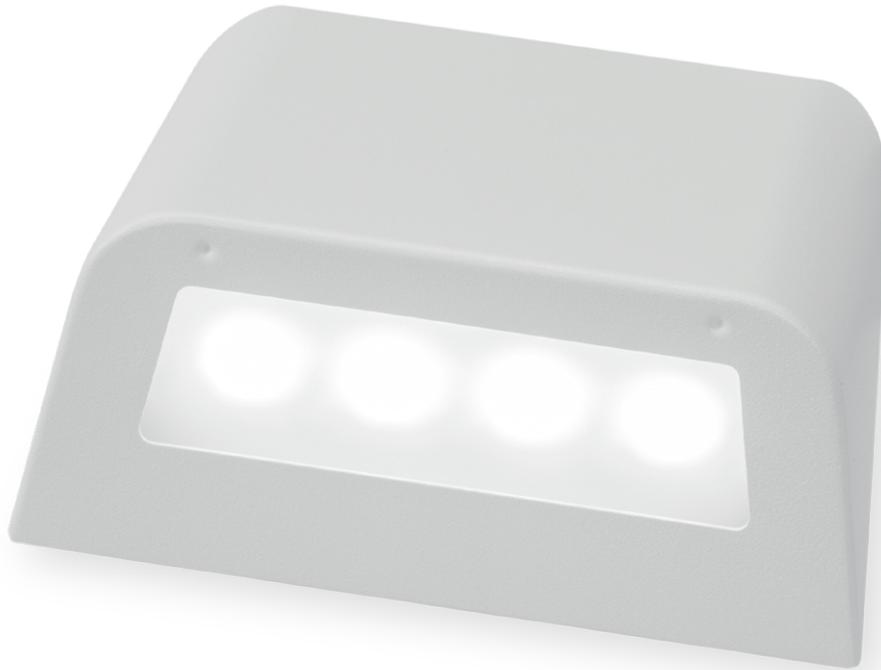
Visually identical, the two luminaires differ in their "interior values": While the PM5 was developed for outdoors (IP65), we have designed the LM5 with a lower degree of protection (IP41). To counteract direct glare, the LED Master LM5/PM5 has a satin finish glass cover, which has an output angle of 45°. Suitable for lighting indoor and outdoor open areas in accordance with EN 1838.
